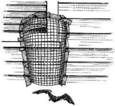
Figure 7-1. One-way doors allow bats to exit a building but prevent their reentry.
