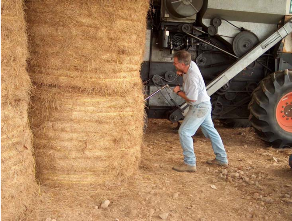
Figure 1. Core samples should be taken from the sides of large round bales.
