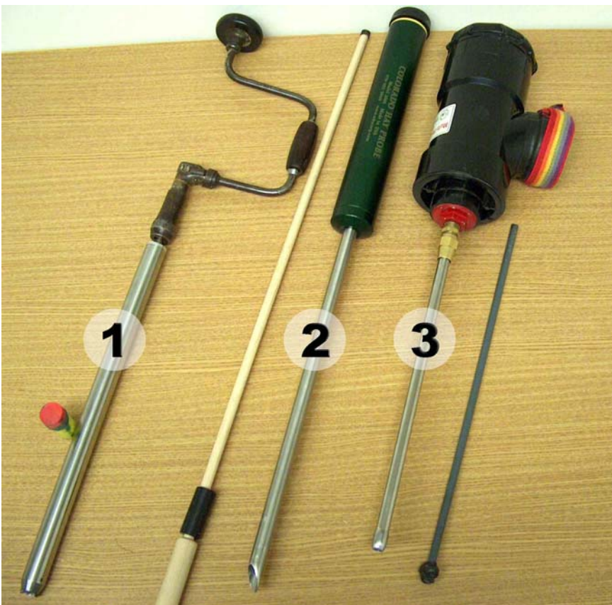
Figure 2. Core sampling devices: (1) Penn State Forage sampler, (2) Colorado Hay Probe and (3) Star Quality Multi-sampler
