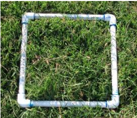
Device used to sample fall armyworm (size: 1 square foot constructed from ½ inch PVC pipe)
